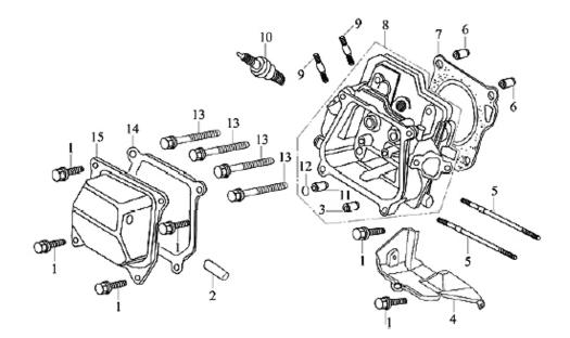
Note: When ordering parts from this list, specify: **Parts List C**, CYLINDER HEAD AND COVER ASSEMBLY and the ITEM No.
